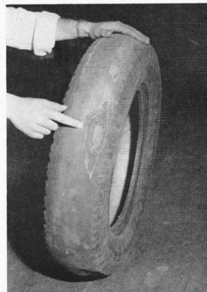
This tire died a premature death because of the owner's neglect. The motorist first failed to change it to other wheels so it would wear down evenly and then he failed to have it recapped in time.
